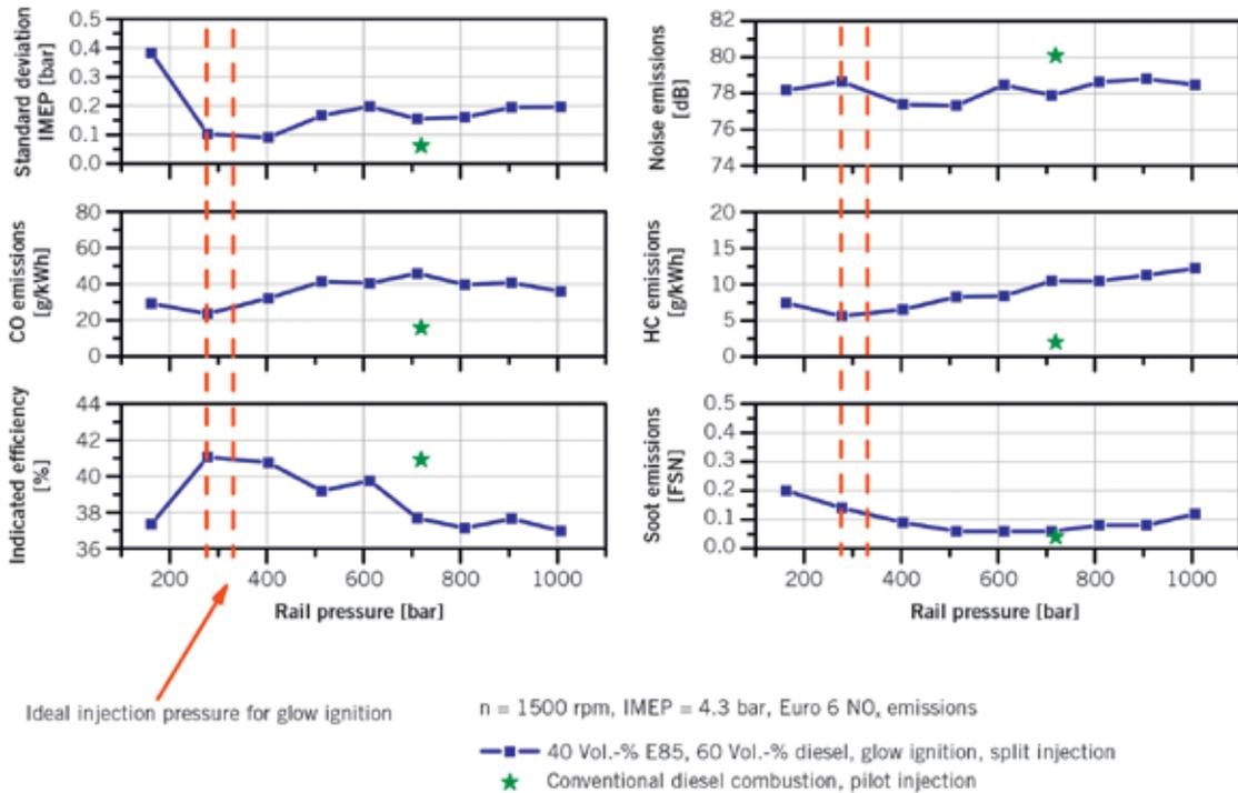
firm the higher stability of glow ignition with decreasing rail pressure. The results from the high pressure chamber can therefore be valuably transferred to diesel engine applications.
