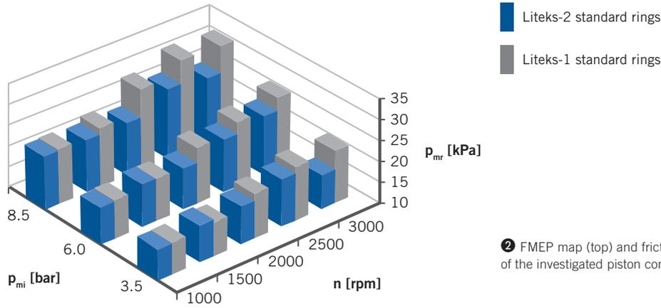
② FMEP map (top) and friction force diagram (bottom) of the investigated piston concepts
