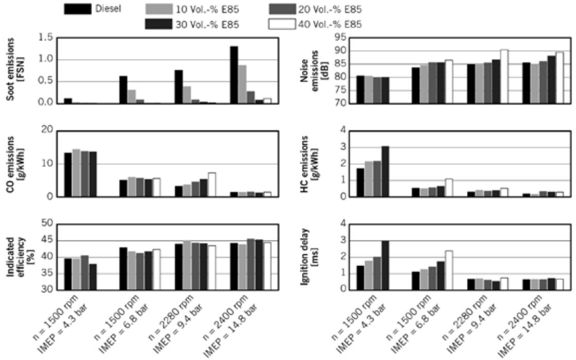
but the advantageous efficiency of the diesel engine's combustion remains even at high ethanol contents.
