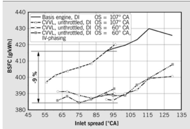
7 The CVVL-engine's brake specific fuel consumption with direct fuel injection at n = 2000 rpm and BMEP = 2 bar
