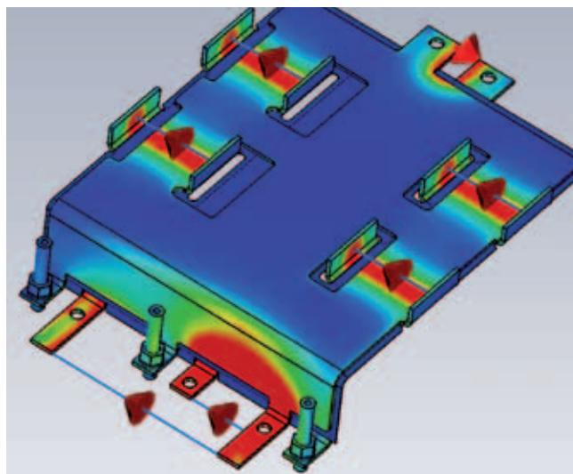
6 Example: visualization of current distribution at a high voltage bus bar
