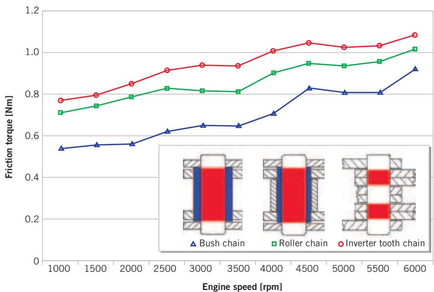
② Friction torque of different chain types (same pitch = 8 mm)
