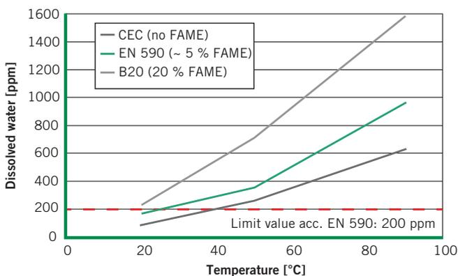
2 Solubility of water in different diesel-biodiesel blends depending on temperature
