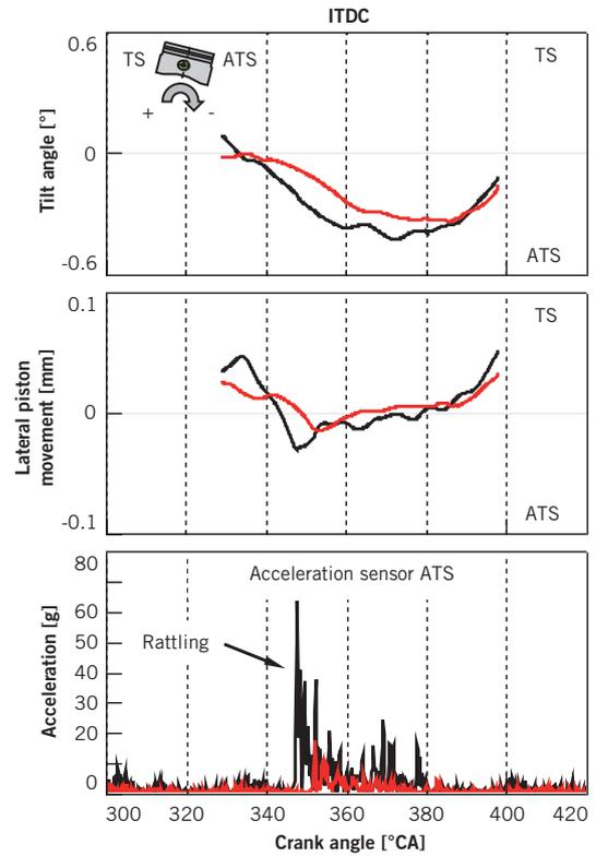
④ Piston motion behaviour with modified skirt stiffness on the thrust side in the bottom skirt area, and anti-thrust-side structure-borne noise excitation, 2400 rpm, 5 Nm, cold engine
