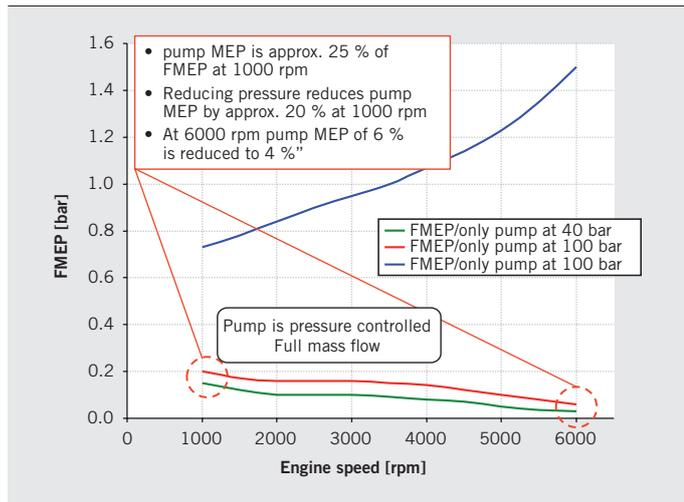
④ Friction mean effective pressure of the fuel pump for high and low pressure
