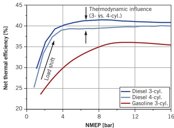
❶ Comparison of the net thermal efficiency between a three- and four-cylinder diesel engine and a three-cylinder gasoline engine with the same displacement ( $V_{disp} = \text{const.} = 1.5 \text{ l}$ )
