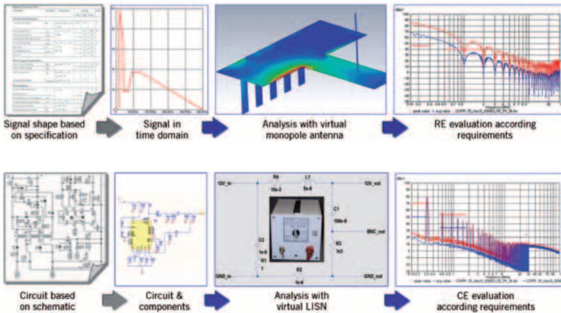
② Example of a requirement based simulation analysis: radiated emission with virtual monopole antenna
