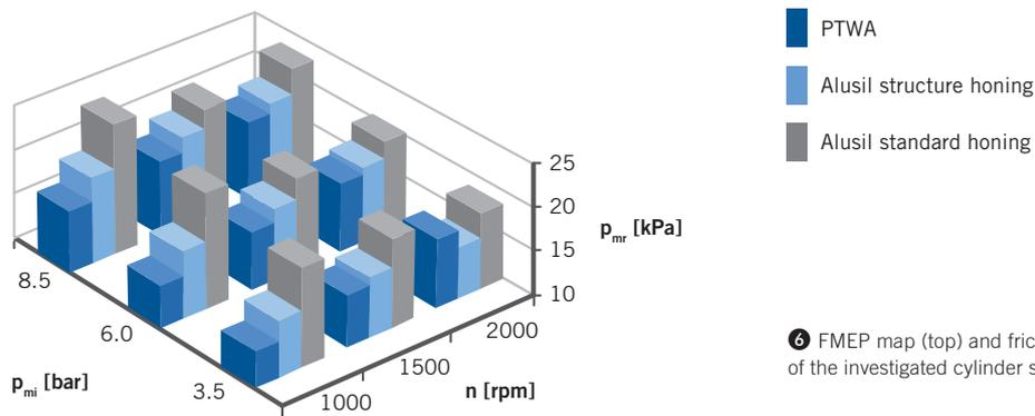
6 FMEP map (top) and friction force diagram (bottom) of the investigated cylinder surface technologies
