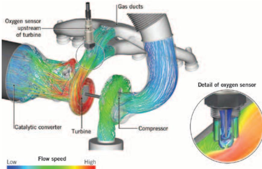
⑤ CFD simulation in the region of the turbocharger (left); detailed calculation of the lambda sensor (right)
