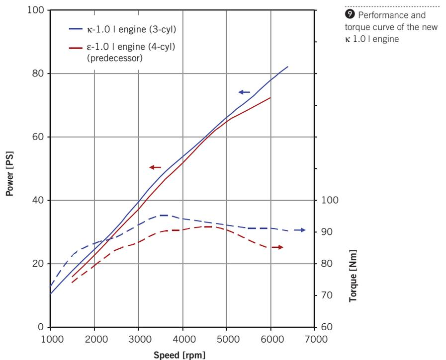
9 Performance and torque curve of the new κ 1.0 l engine
