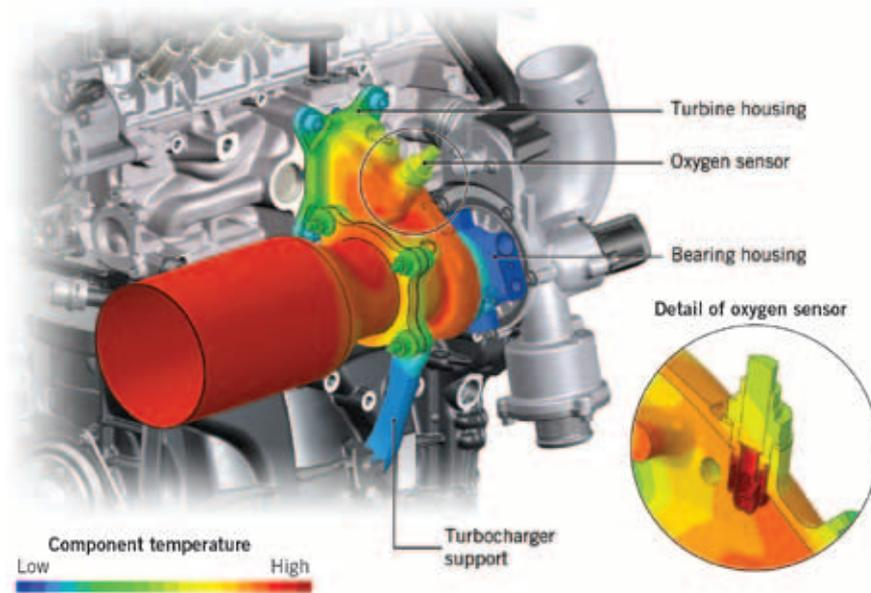
⑥ FEM simulation of the turbocharger and detailed calculation of the lambda sensor (temperature distribution)
