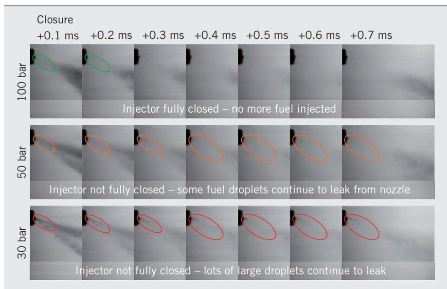
1 Injector closing at different injection pressure
