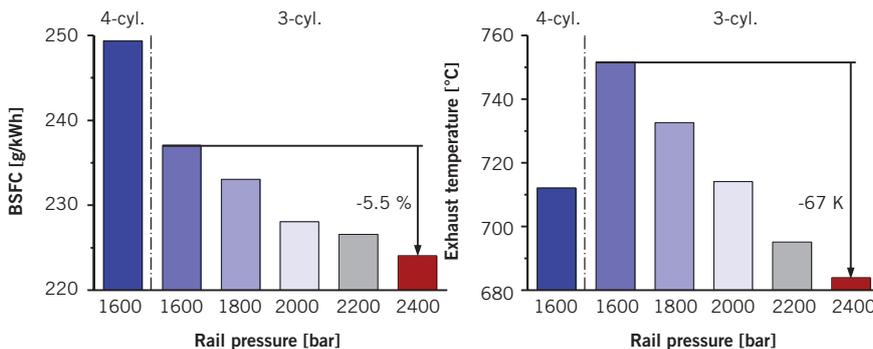
⑥ Rail pressure variation at rated power of the four-cylinder engine
