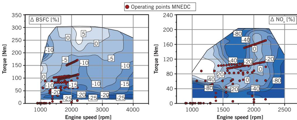
③ Deviation (BSFC and NO<sub>x</sub> emissions) between three- and four-cylinder engine
