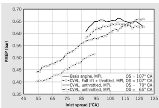
④ PMEP over inlet spread at  $n = 2000$  rpm und  $BMEP = 2$  bar
