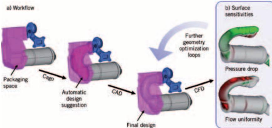
6 a) Workflow for catalyst cone development, b) surface sensitivities for subsequent geometry optimization
