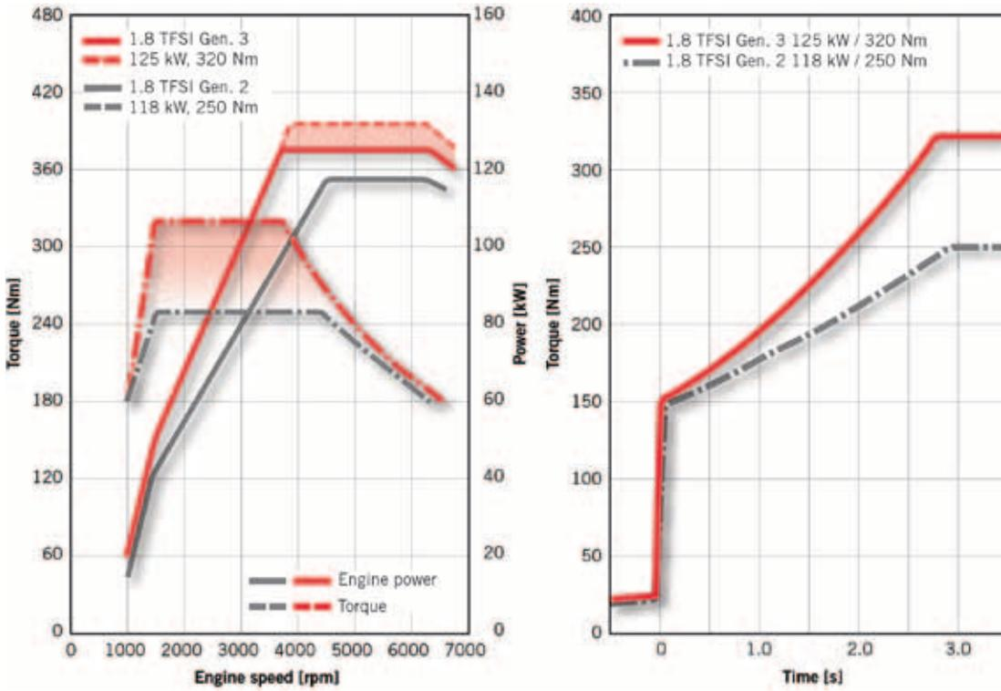
with the second-generation 2.0 l EA888 engine with the Audi valvelift system (132 kW/320 Nm), there is still a clear, 14 % improvement in fuel consumption, with the same performance.
