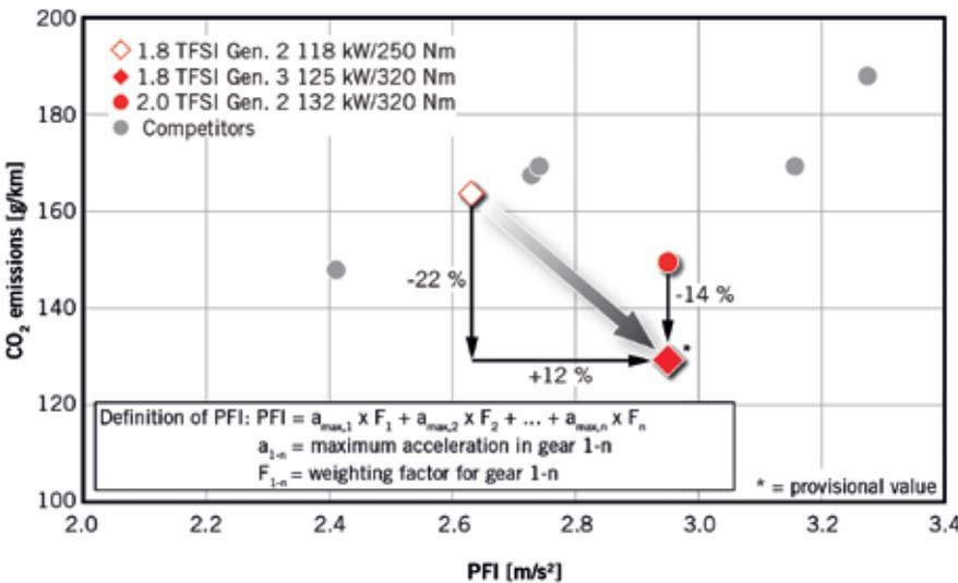
8 CO<sub>2</sub> emissions versus performance (PFI – performance feel index, weighted average acceleration ability in all gears)
