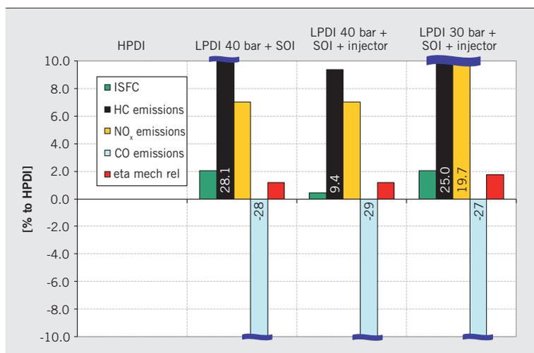
⑦ Experimental results 5000 rpm and 10 bar BMEP
