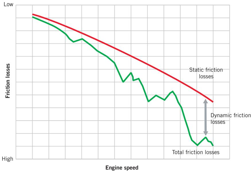
① Calculated friction losses
