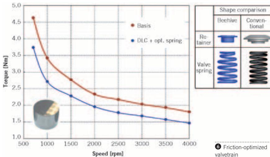
curved structure from the typical straight variety, which improves torque and maximum power by 1.0 Nm and 1.5 kW,
