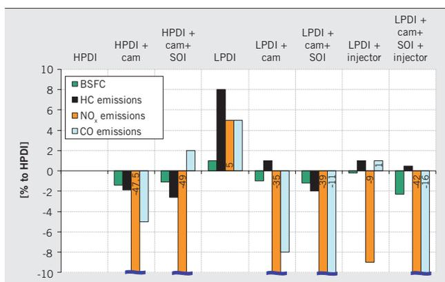
5 Experimental results 2000 rpm and 2 bar BMEP
