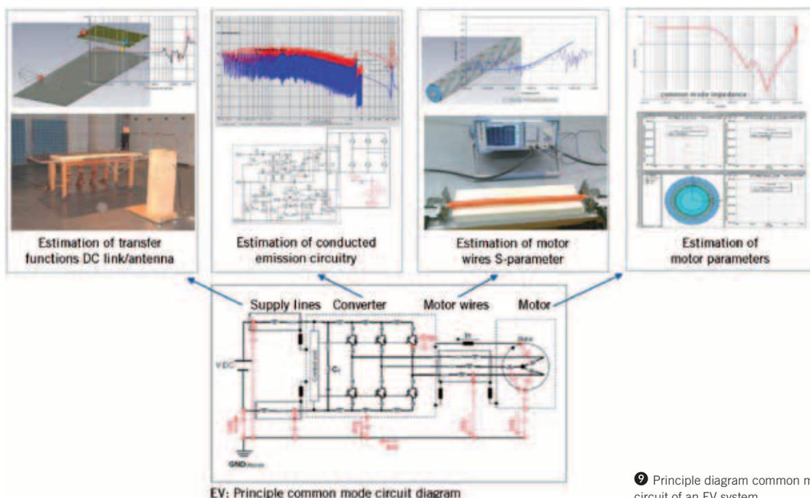
9 Principle diagram common mode circuit of an EV system
