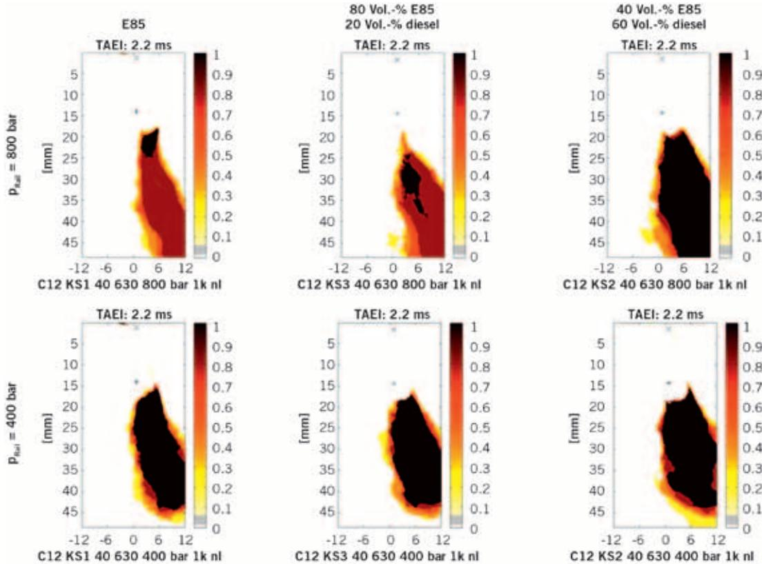
⑥ Probability distribution of light emitted by the flame for experiments carried out with E85 and E85 diesel mixtures at injection pressures of 800 bar and 400 bar
