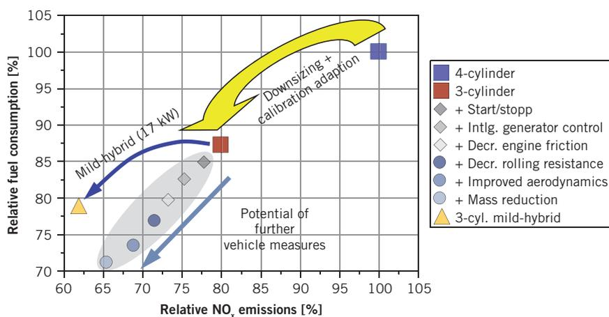
9 Potentials of vehicle measures and mild-hybrid for further decreasing of fuel consumption and nitrogen oxide emissions
