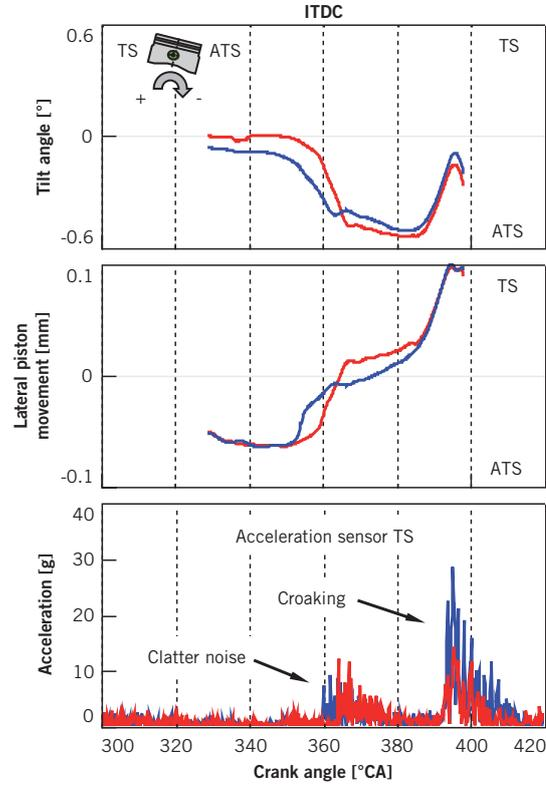
③ Piston motion behaviour with modified skirt stiffness on the antithrust side in the top skirt area, and thrust-side structure-borne noise excitation, 1600 rpm, 50 Nm, cold engine
