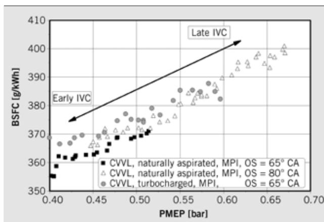
⑤ Specific fuel consumption over PMEP at  $n = 2000$  rpm und  $BMEP = 2$  bar
