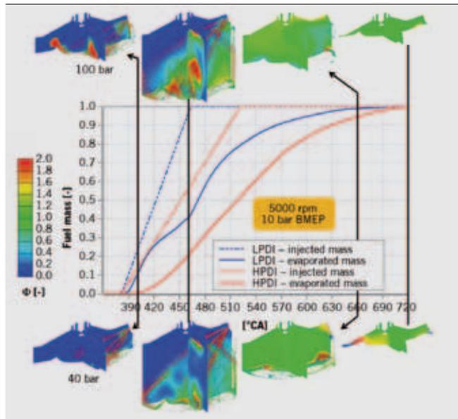
② Comparison of mixture formation for high and low pressure injection
