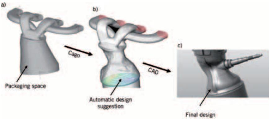
5 Catalyst inlet cone for four-cylinder naturally aspirated engine
