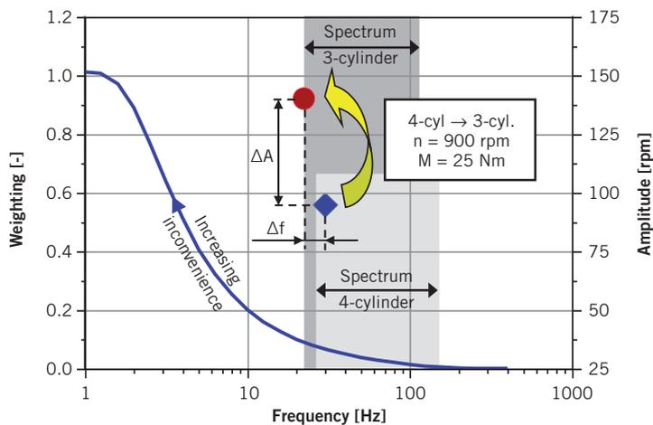
8 Engine vibrations of three- and four-cylinder engines and their inconvenience level
