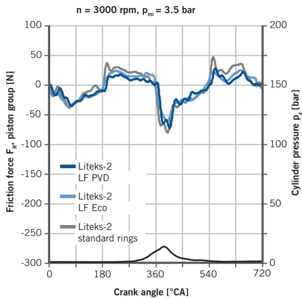
demonstrated in the ring simulation are depicted in the partial load characteristic map. This reveals the friction advantages in FMEP for all operating points starting with a speed of 1500 rpm. Depending on the operating point, with the LF Eco these can amount to 10 % and 22 %, and with the LF PVD, to between 26 % and 37 %.
