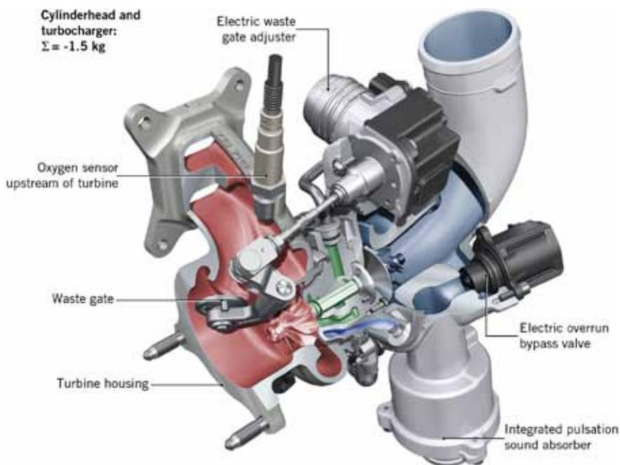
④ Compact turbocharger module with lambda sensor ahead of the turbine and electric wastegate actuator
