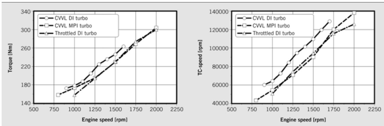
③ Comparison between the torque and the ATL-engine speed of the different engine concepts at full load
