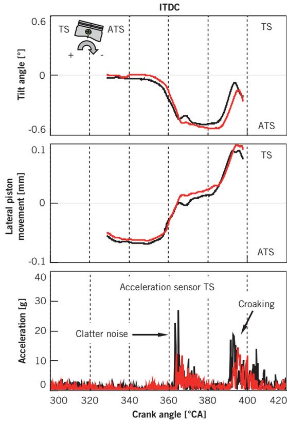
5 Piston motion behaviour with modified skirt stiffness on the thrust side in the bottom skirt area, and thrust-side structure-borne noise excitation, 1600 rpm, 50 Nm, cold engine
