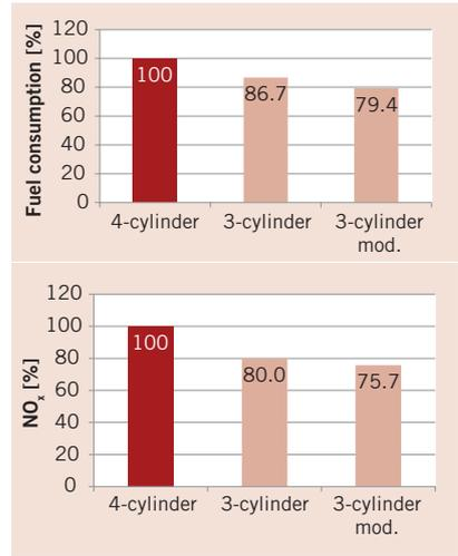
② Specifications of the modified downsizing engine; reduction of fuel consumption and nitrogen oxides in the MNEDC, measured on the chassis dynamometer
