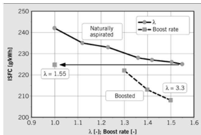
② Specific fuel consumption with varying the air-fuel ratio and the boost rate [14] at  $n = 2000$  rpm und  $IMEP = 7$  bar
