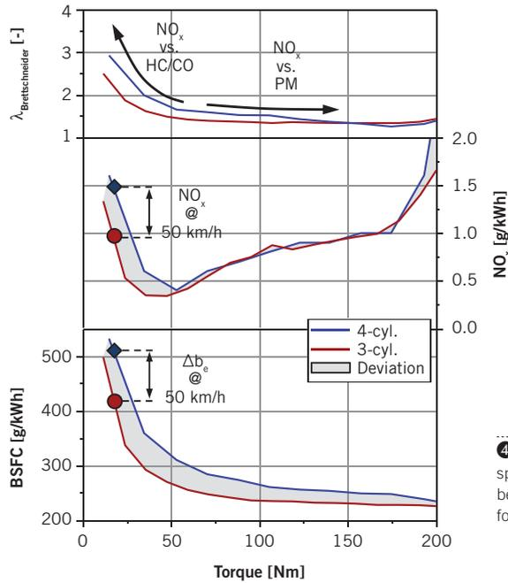
④ Comparison of air-to-fuel ratio, specific  $\text{NO}_x$  emissions and BSFC between three- and four-cylinder engine for a load sweep at 2000 rpm
