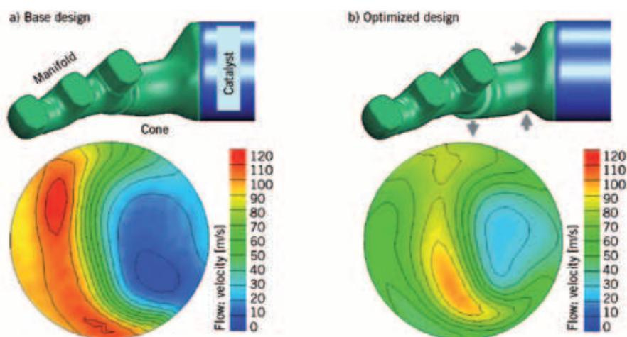
❶ Closed coupled catalyst and a three-in-one manifold of a twelve-cylinder engine
