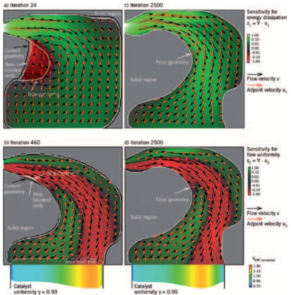
③ Sensitivities for backpressure in inlet cone (a, c) and for flow uniformity across the catalyst (b, d) after 24 iterations (a), after 460 iterations (b) and after 2500 iterations (c, d); final cone geometry after 2500 iterations (c, d)
