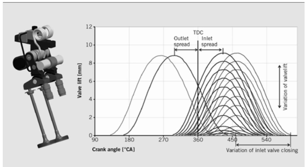
inlet spread (IS) or the inlet valve lift and in the case of the outlet side the outlet spread (OS). The fixed relation between valve lift and timing can be uniquely configured at the valve drive's arrangement.
