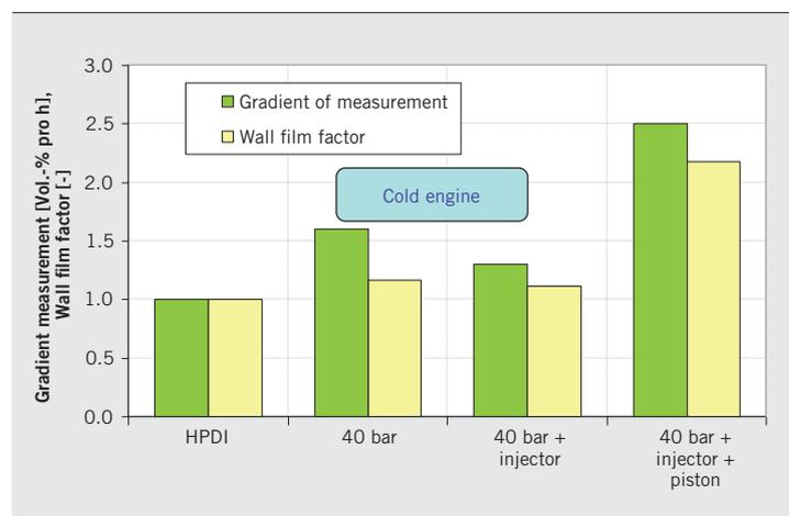
⑧ Comparison of simulation and measurement gradient of oil dilution
