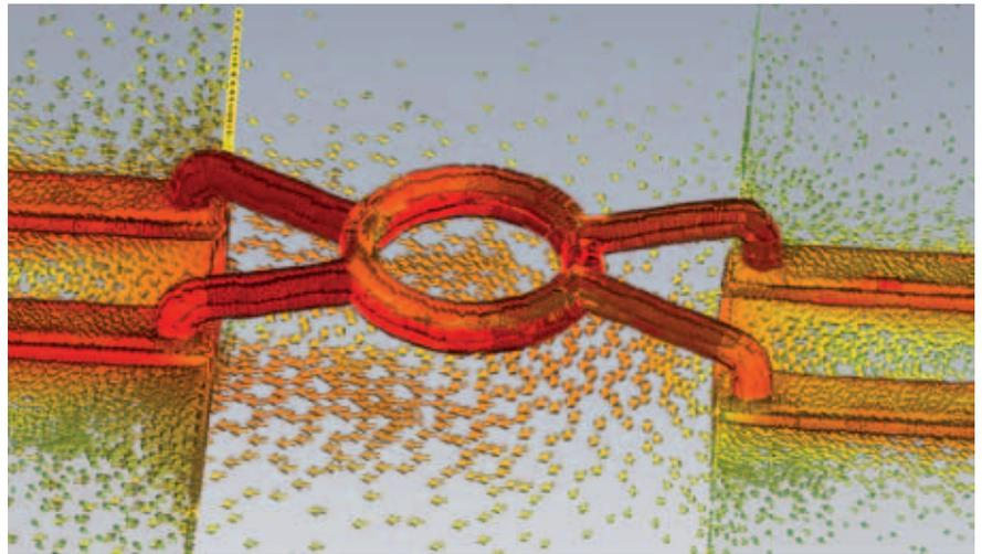
5 Example: visualization of eddy currents in a metal structure cause by a transformer
