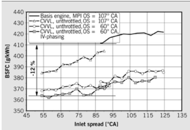
6 Brake specific fuel consumption of the CVVL-engine with port fuel injection at n = 2000 rpm und BMEP = 2 bar
