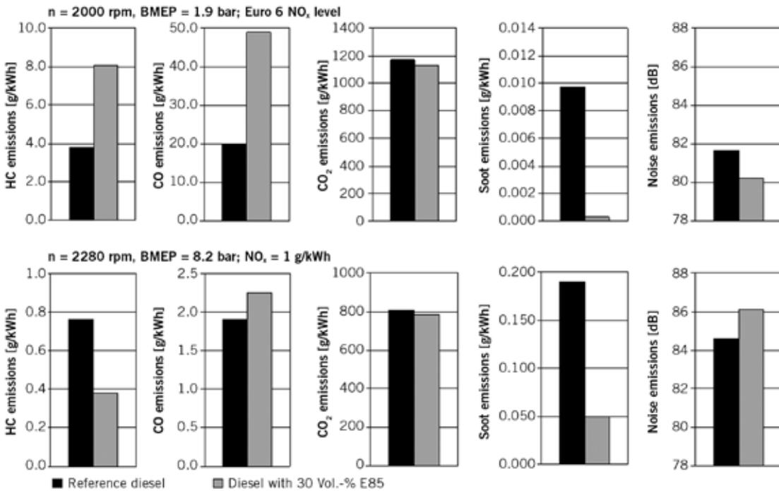
5 Comparison of emission results in a multi-cylinder engine, with pilot injection and constant center of combustion
