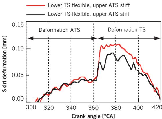
6 Dynamic piston skirt deformation at the height of the lower measuring plane, during operation at 1600 rpm and 50 Nm, cold engine
