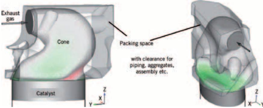
4 Automatically generated inlet cone for the provided packaging space
