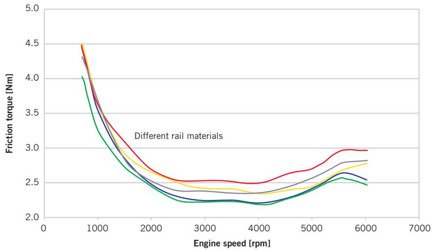
④ Chain drive friction losses
